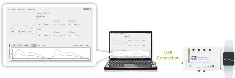
Figure 11: SpO 2 Test Mode Product Wiring Diagram
