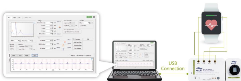
Figure 7: ECG Test Mode Product Wiring Diagram
