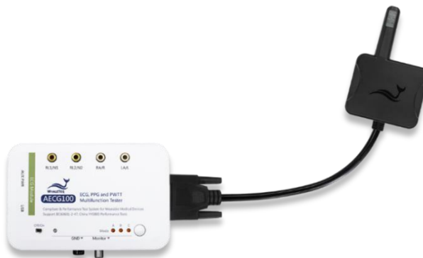
Figure 6: Direct Connection between AECG100 and PPG-2TF-660
