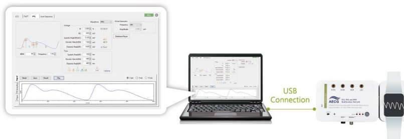
Figure 9: PPG Heart Rate Test Mode Product Wiring Diagram
