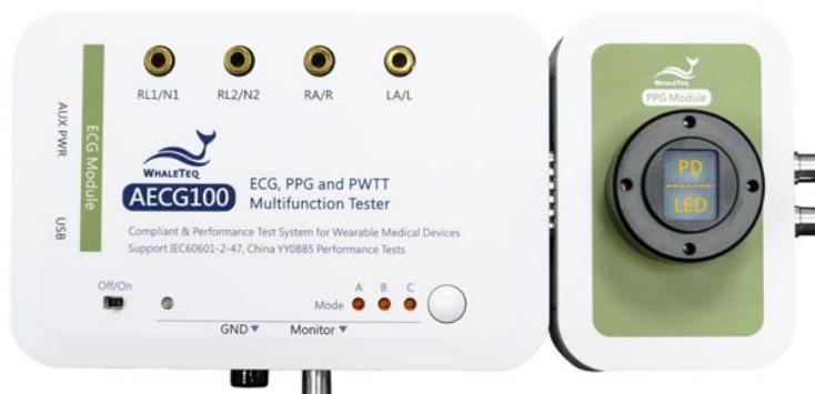
Figure 4: Direct Connection between AECG100 and PPG Module
